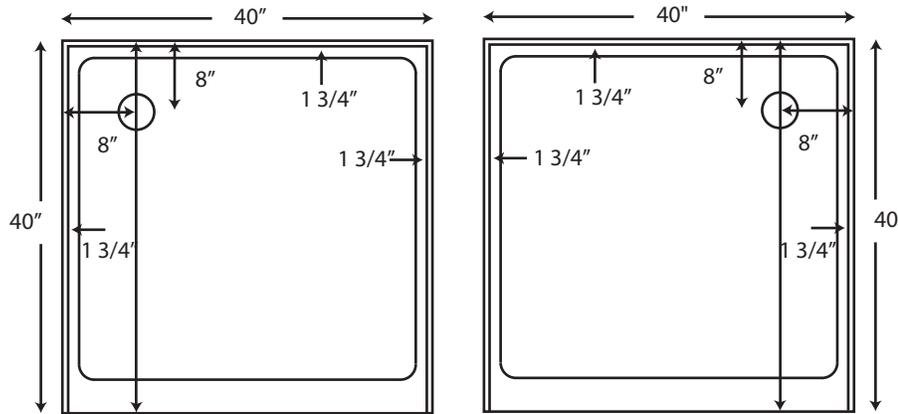
**Note: Drain opening is NOT a standard drain opening. This base can only be used with the Winglts Vortex Shower Drain pictured below.**
