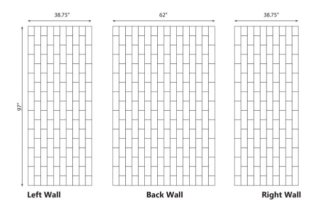
FEATURES Dimensional Tolerance ± 1/8". Dimensions needed for site preparation should be measured from the unit. American Bath Group assumes no responsibility for preparatory work.
