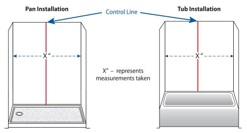
3. **Cutting the back surround to fit:** Using your CL as your guide, you will measure from the top of the shower pan / tub up to the CL on the back wall on the left side, right side, and middle. You will also measure from the top of the shower pan / tub to the ceiling in the same three locations. Always cut the panels from the top (color side) using a circular blade cutting down on the panel.
