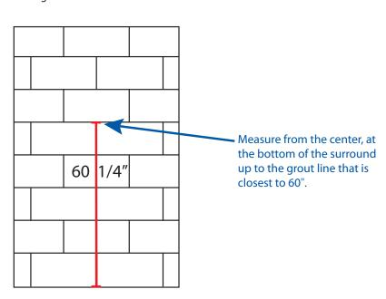
Take the grout line measurement you took on the Tub / Shower Surround and subtract a half inch:  $60 \frac{1}{4}" - \frac{1}{2}" = 59 \frac{3}{4}"$ . Measure from the top of the shower pan, at the center, going vertically measure up to  $59 \frac{3}{4}"$  and mark. Using a level draw your control line across the back wall.
