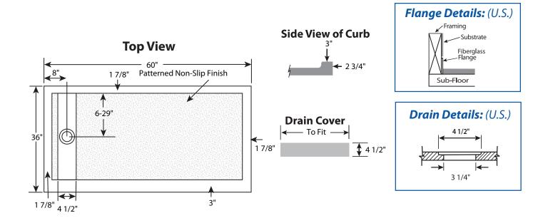
$\textbf{FEATURES} \ \ \textbf{Dimensional Tolerance} \ \pm 14\text{".} \ \textbf{Dimensions needed for site preparation should be measured from the unit.} \ \textbf{American Bath Group assumes no responsibility for preparatory work.}$
