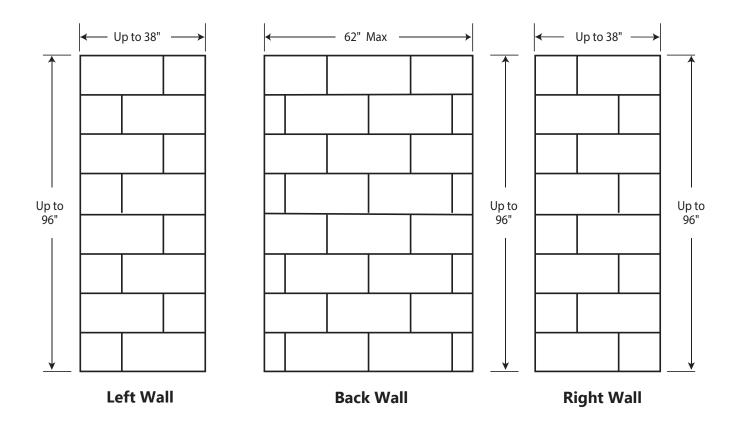
$FEATURES \quad \text{Dimensional Tolerance} \pm \frac{1}{4}\text{". Dimensions needed for site preparation should be measured from the unit. American Bath Group assumes no responsibility for preparatory work.}$
