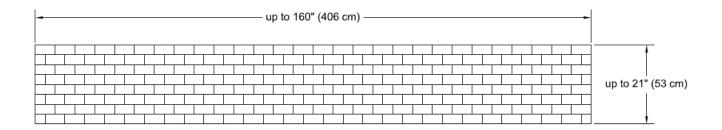
FEATURES Dimensional Tolerance ± 1/4". Dimensions needed for site preparation should be measured from the unit. American Bath Group assumes no responsibility for preparatory work.
