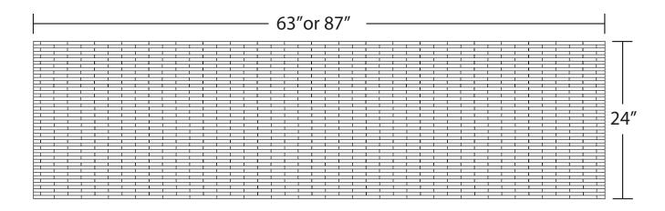
FEATURES Dimensional Tolerance  $\pm \frac{1}{4}$ ". Dimensions needed for site preparation should be measured from the unit. American Bath Group assumes no responsibility for preparatory work.
