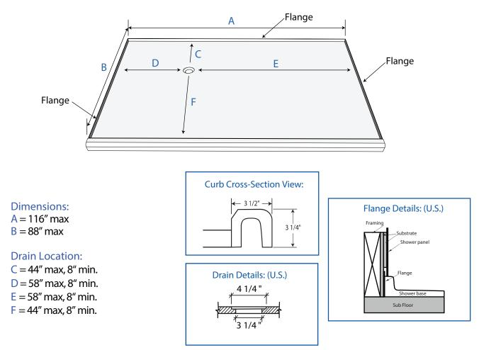
FEATURES Dimensional Tolerance ± 1/4"Dimensions needed for site preparation should be measured from the unit. American Bath Group assume no responsibility for preparatory work.
