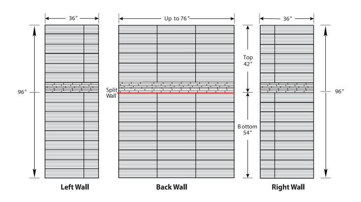
$\label{lem:propagation} FEATURES \ \ \ Dimensional\ \ Tolerance \pm \frac{1}{4}". Dimensions needed for site preparation should be measured from the unit. American Bath Group assumes no responsibility for preparatory work.$
