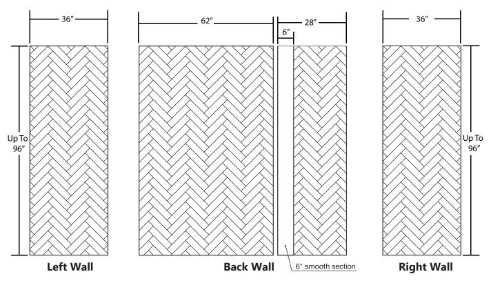
\*The 62" back wall can be trimmed to accommodate a 72" or larger wall up to 88"
