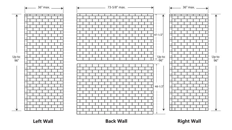
FEATURES Dimensional Tolerance  $\pm \frac{1}{4}$ ". Dimensions needed for site preparation should be measured from the unit. American Bath Group assumes no responsibility for preparatory work.
