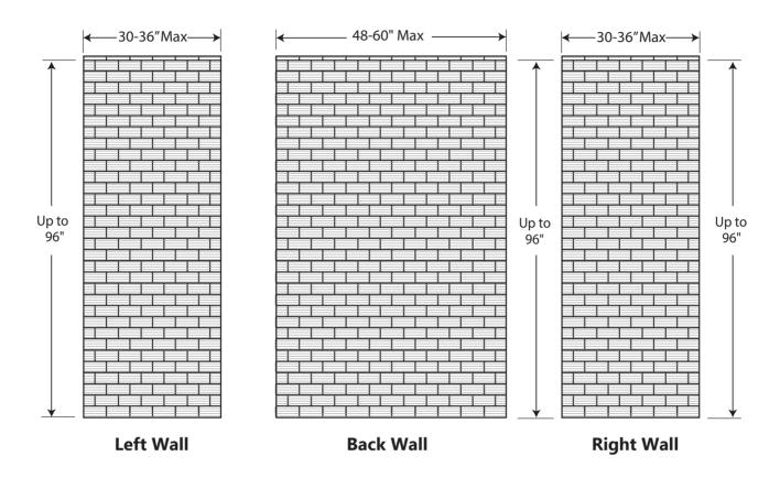
FEATURES Dimensional Tolerance ± 1/4" . Dimensions needed for site preparation should be measured from the unit. American Bath Group assumes no responsibility for preparatory work.
