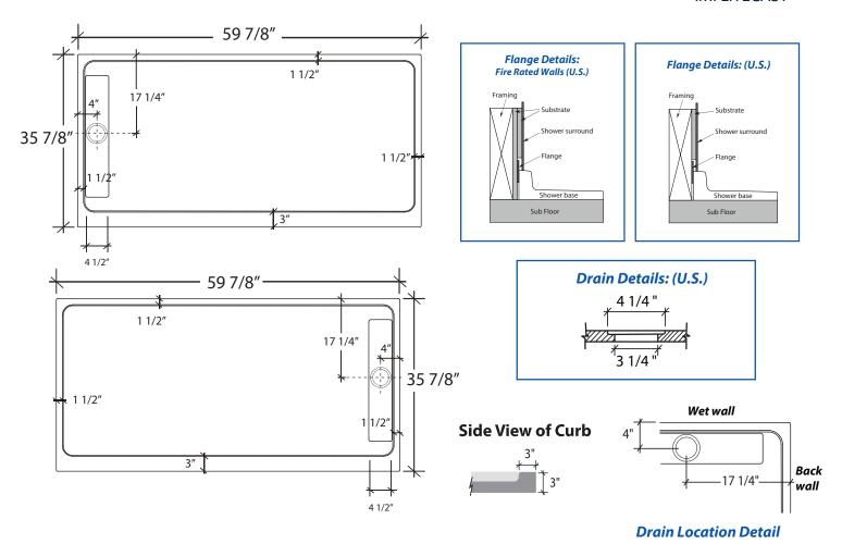
$FEATURES \ \ Dimensional\ Tolerance \pm \frac{1}{4}". Dimensions\ needed\ for\ site\ preparation\ should\ be\ measured\ from\ the\ unit.\ American\ Bath\ Group\ assumes\ no\ responsibility\ for\ preparatory\ work.$
