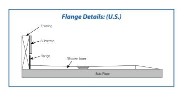
$FEATURES \ \ Dimensional \ Tolerance \pm 1/4". \ Dimensions \ needed \ for \ site \ preparation \ should \ be \ measured \ from \ the \ unit. \ American \ Bath \ Group \ assumes \ no \ responsibility \ for \ preparatory \ work.$
