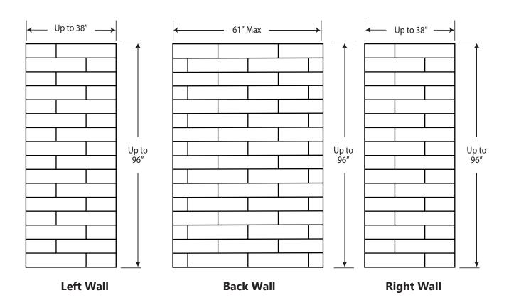
FEATURES Dimensional Tolerance ± ¼". Dimensions needed for site preparation should be measured from the unit. American Bath Group assumes no responsibility for preparatory work.
