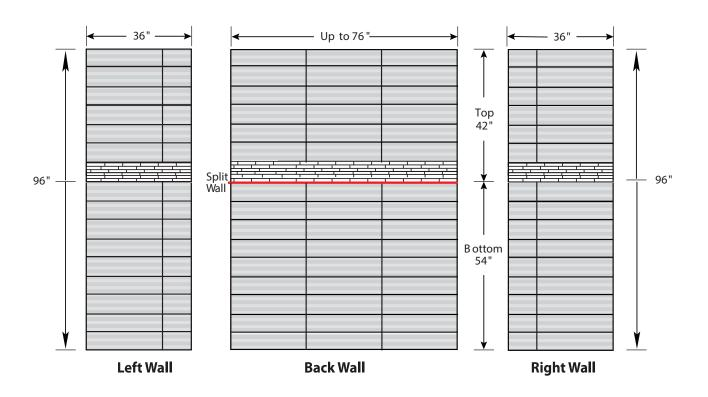
$\label{eq:FEATURES} \textbf{ Dimensional Tolerance} \pm \frac{1}{4} \text{"}. \textbf{ Dimensions needed for site preparation should be measured from the unit. American Bath Group assumes no responsibility for preparatory work.}$
