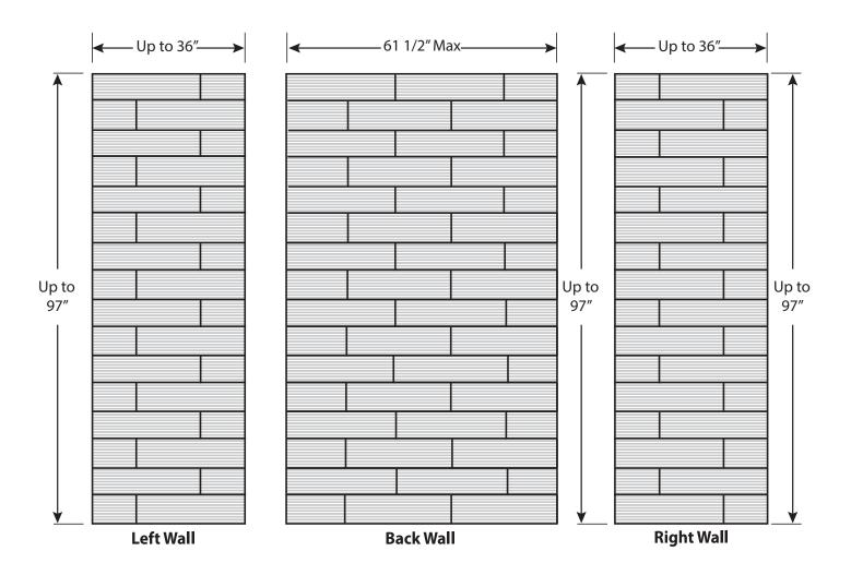
$FEATURES \quad \text{Dimensional Tolerance} \pm \frac{1}{4}\text{". Dimensions needed for site preparation should be measured from the unit. American Bath Group assumes no responsibility for preparatory work.}$
