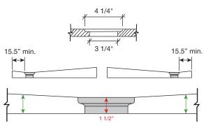
\*The threshold thickness will vary to accommodate the slope needed for proper drainage
