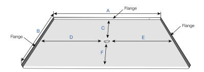
\* The threshold thickness will increase progressively as it extends away from the drainage point. The threshold height on either side may vary depending on the client's preferred drain location.
