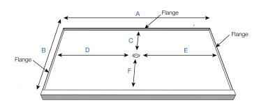
\* The threshold thickness will increase progressively as it extends away from the drainage point. The threshold height on either side may vary depending on the client's preferred drain location.
