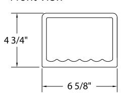
FEATURES Dimensional Tolerance ± 1/8". Dimensions needed for site preparation should be measured from the unit. American Bath Group assumes no responsibility for preparatory work.
