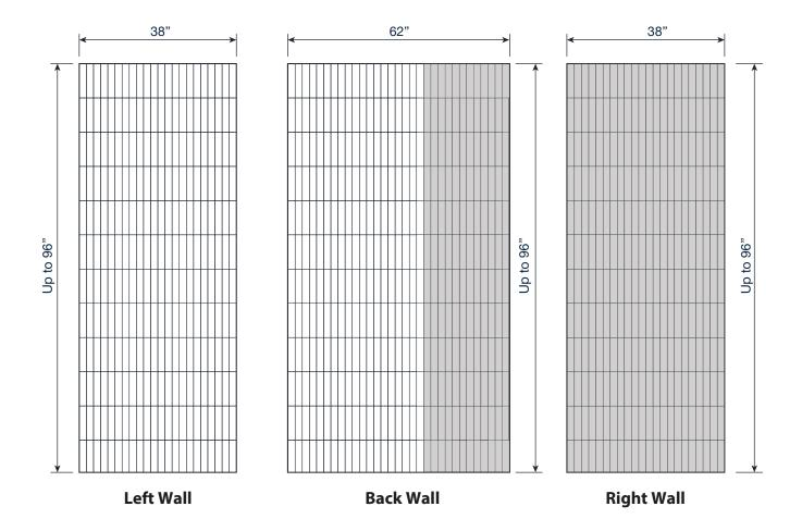
$FEATURES \ \ Dimensional\ Tolerance \pm 1/4". Dimensions\ needed\ for\ site\ preparation\ should\ be\ measured\ from\ the\ unit.\ American\ Bath\ Group\ assumes\ no\ responsibility\ for\ preparatory\ work.$
