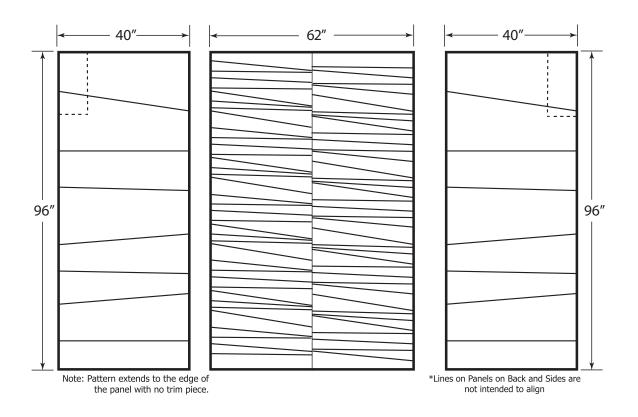
$\textbf{FEATURES} \ \ \text{Dimensional Tolerance} \ \pm 1/4\text{"}. \ \text{Dimensions needed for site preparation should be measured from the unit.} \ \ \text{American Bath Group assumes no responsibility for preparatory work.}$
