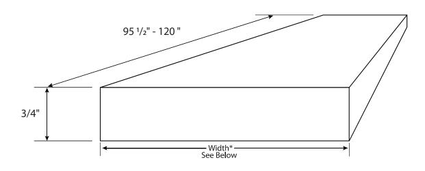
$FEATURES {\it Dimensional Tolerance} \pm 1/8". Dimensions needed for site preparation should be measured from the unit. American Bath Group assumes no responsibility for preparatory work.$
