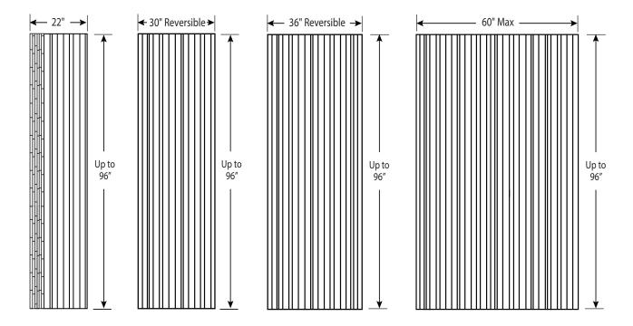
$FEATURES \quad \text{Dimensional Tolerance} \pm \frac{1}{4}\text{". Dimensions needed for site preparation should be measured from the unit. American Bath Group assumes no responsibility for preparatory work.}$
